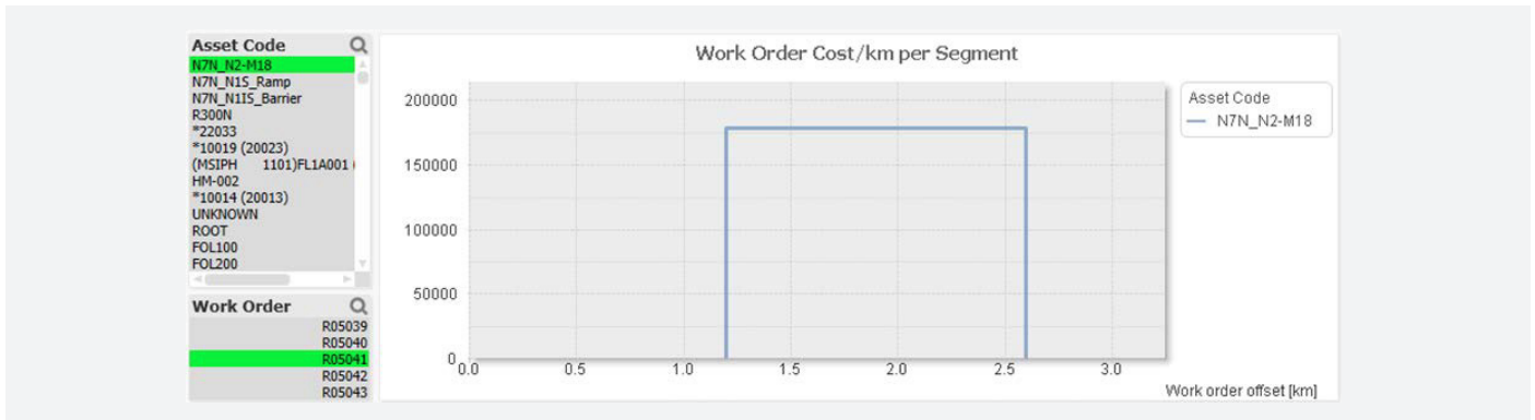
Fig. 6. Work order R05041 shown to contribute significantly to maintenance cost of the N7N_N2-M18 road section.
